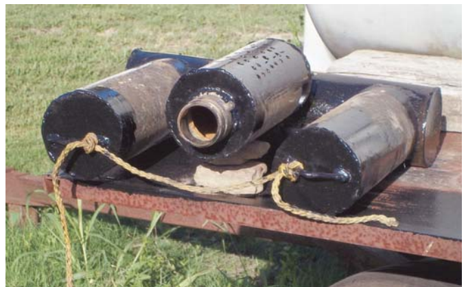
Float is made up of three 2-ft. long metal tubes welded together, with a fourth tube at the center that pivots on a metal pin so tube can move up and down.
