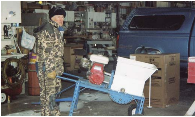
Ron Hein's homemade mini hammermill can be moved around by hand using drop down handles.
