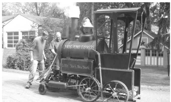
Tino Ferro made this miniature version of an old steam engine from memory. It’s powered by a 6 1/2 hp motor and can go about 8 mph.
