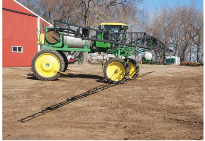
Front-mounted boom is based on commercial booms and has 5-ft. breakaways at either end.
