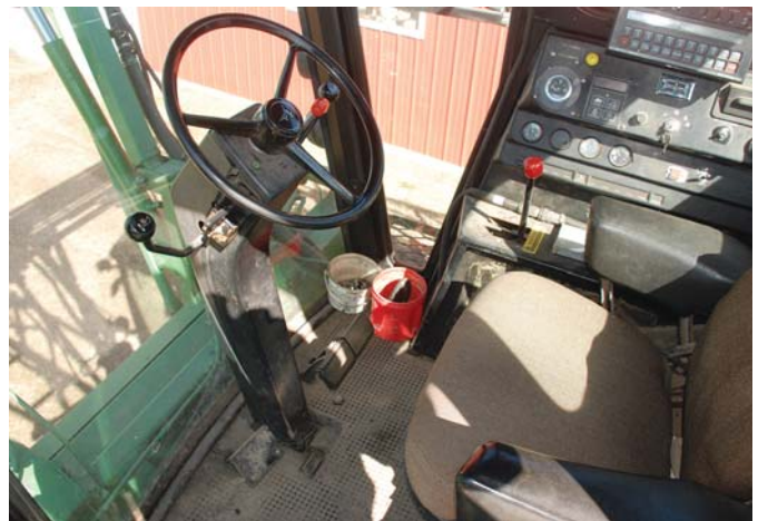
Flipping between the two steering modes is as simple as stepping on a clutch-type pedal on the cab floor.
