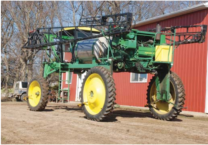
Articulated steering lets sprayer's rear wheels exactly track the front wheels on end rows. When desired, the articulation joint locks and front-wheel steering takes over.
