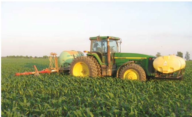
Jeff Wuebker built this 12-row, side dress rig that's equipped with 500-gal. tanks front and back. A cantilevered center beam holds front tank in place.
