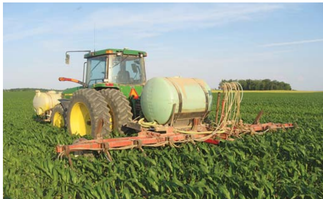
Rear tank sits on frame mounted on his Deere 8440's 3-pt. hitch.
