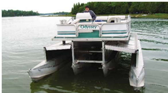
Pontoon boat with extra set of pontoons is designed to ride smoothly through waves up to 4 ft. high with minimal bounce.
