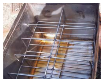
Canner is divided by a stainless steel rack that sets inside the container.
