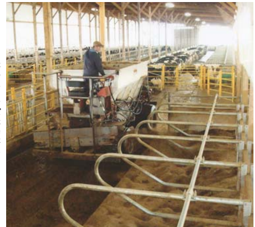
George Edmond built this sand shooter to bed cow stalls with sand. The self-propelled cart can empty a 7 cu. yd. box of bedding sand in just 5 min., shooting the sand up to 10 ft. out from the cart.
