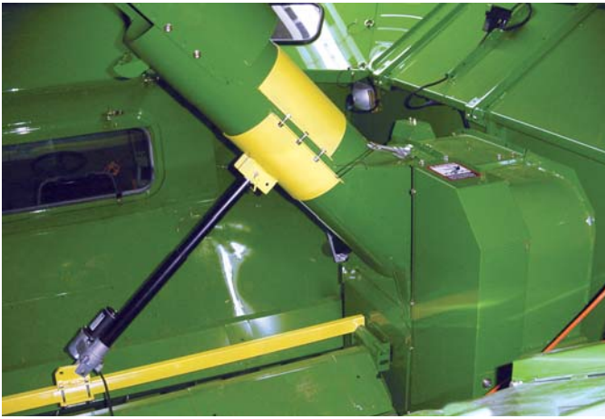
Add-on kit lets you lower the bin auger on a Deere 9600 Series combine by simply pressing a switch.
