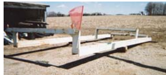
To convert the flatbed Dittmer simply backs the trailer with dovetail under the subframe, which slides up and over the trailer deck.
