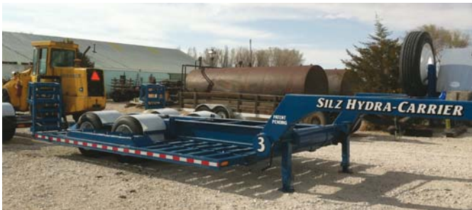
Remote-controlled trailer is equipped with an electric/hydraulic power system and a hinging system that folds in the sides and ramps.
