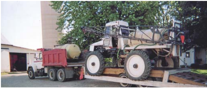
Gene Dittmer added a subframe to an old flatbed trailer, allowing it to hold his wide wheel track sprayer. Subframe can be easily removed to haul his backhoe.
