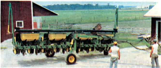
The planter transport requires no modification of planter. Attaches to frame with four bolts.
