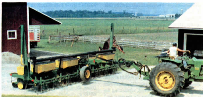
Telescoping gooseneck lengthens to pull planter in-line behind the tractor.
