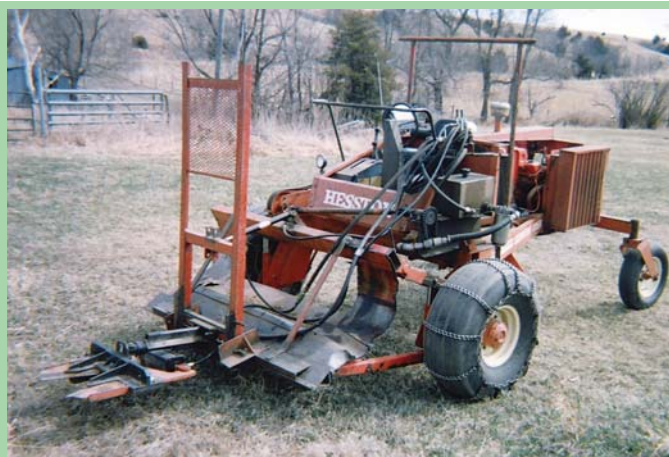
To build his low-cost tree cutter, Ben Stuppelbeen mounted a Precision tree shear on front of a Hesston swather.
