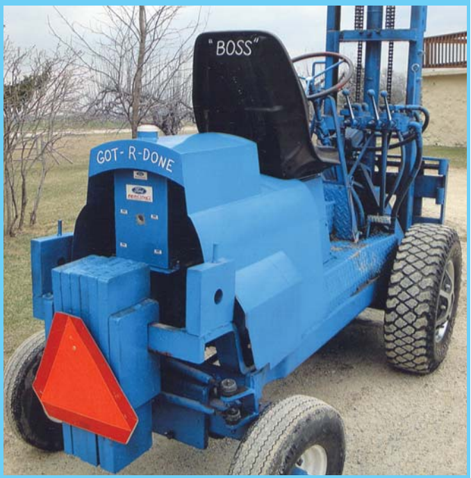
A series of 24-in. long weights on back counteract weight of mast load.
