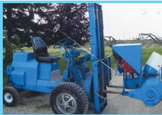
Big snowblower fits onto fork tines, Odenwald rigged up a small wheel to turn snowplow.
