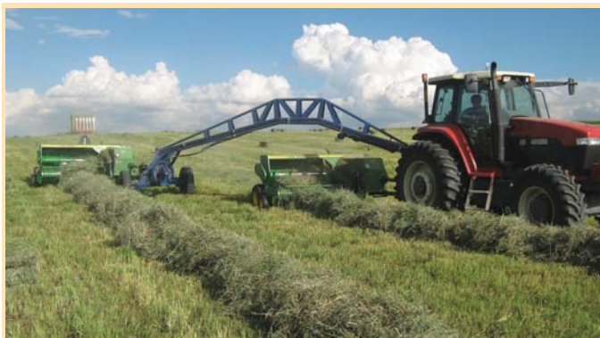
Dale and Richard Hallett built this double hitch for their small square balers. Connecting arch contains no gearboxes or driveshafts, only hydraulic hoses.
