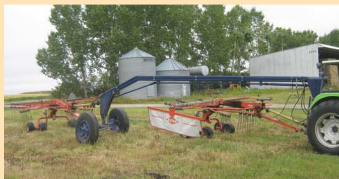
The Halletts also built this double rake hitch. Second rake is pulled by a 2-wheel cart attached to a 20-ft. length of sq. tubing that arches over the first rake.
