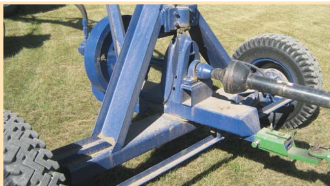
Arch attaches to cart axle with an A-frame. Second baler's pto drive is powered by a hydraulic motor.
