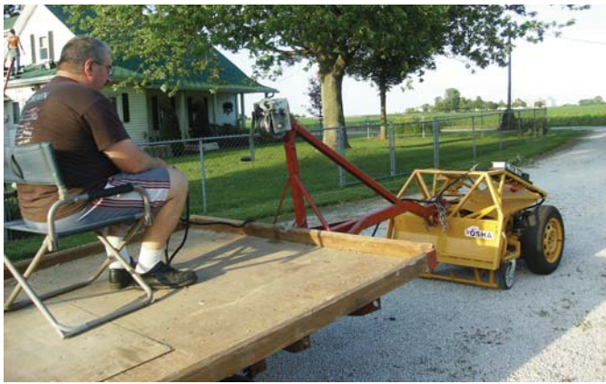
Self-propelled robotic tug can easily tow 10 adults on a trailer at 2 1/2 mph, says inventor Roy Visser.
