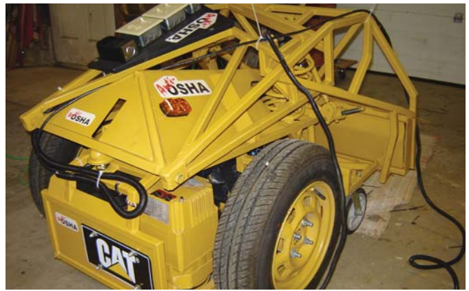
Power for the tug is provided by an engine-driven generator. Power tools can be plugged into a pair of 110 and 220-volt outlets.
