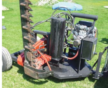
Canadian researcher Richard Grosshans built this cattail harvester that's towed by an 8-wheel Argo amphibious vehicle.
