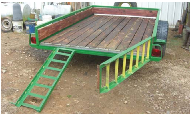
A pair of ramps also form trailer's tailgate. To the trailer's fenders, Zenz used tires cut in half.
