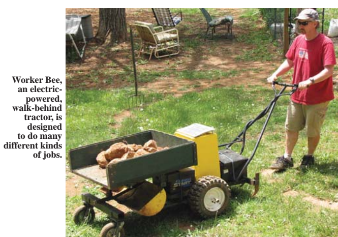
Unit can be used with a bucket to scoop dirt or snow (left) or to operate a self-dumping power wheelbarrow.
