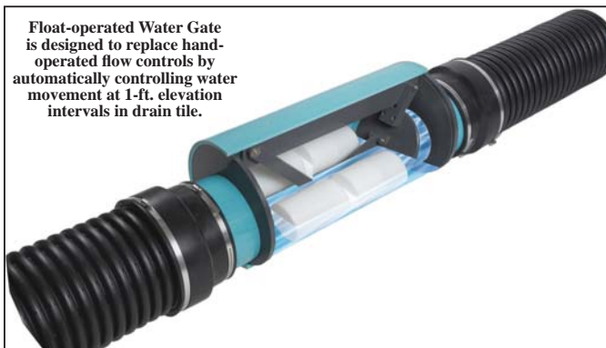
Unit opens and closes based on water levels downstream.
