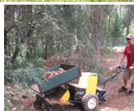
Unit can be used with a bucket to scoop dirt or snow (left) or to operate a self-dumping power wheelbarrow.
