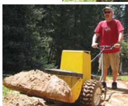
Unit can be used with a bucket to scoop dirt or snow (left) or to operate a self-dumping power wheelbarrow.
