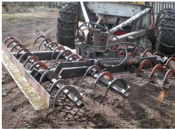
Bale handling forks have a pivot point at center that allows Siddoway to stack bales lengthwise and crosswise for a more stable load.
