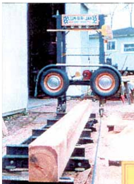
Reek's first sawmill, the Lum-BR-Jak, was built in 1994 from miscellaneous parts for less than $100.
