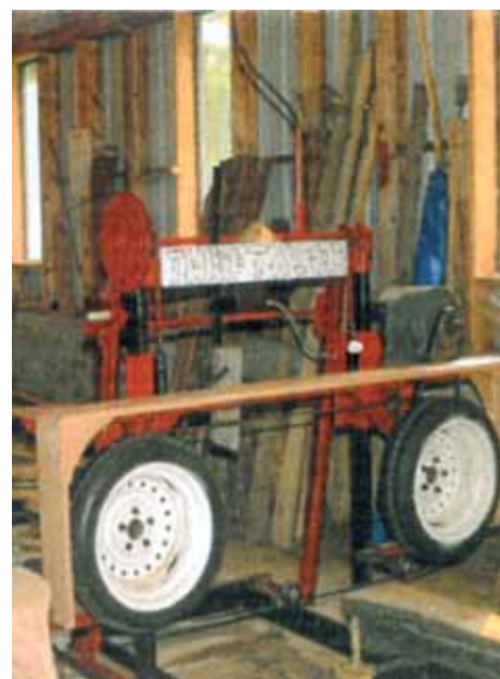
In 2010 Reeks designed his latest new sawmill, the Thriftwood. It's powered by a single phase 220-V motor. No fumes so it can be used inside.
