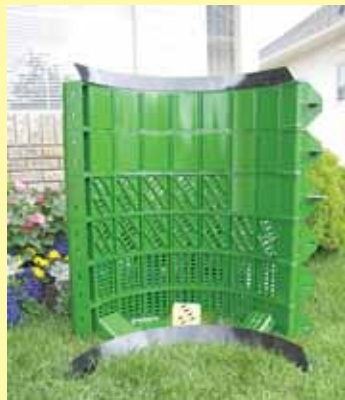
Photo (above) shows 6 frames with 3 different kinds of modules - 2 Minimum Thresh at the top, 2 Maximum Thresh in the middle, and two 21-Hole standards at the bottom. Photo below shows how modules fit into frame.
