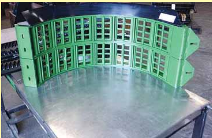
Instead of large, full-size concave panels, Sunnybrook Welding offers frames that each hold individual modules. Modules in this frame are designed for peas and beans.
