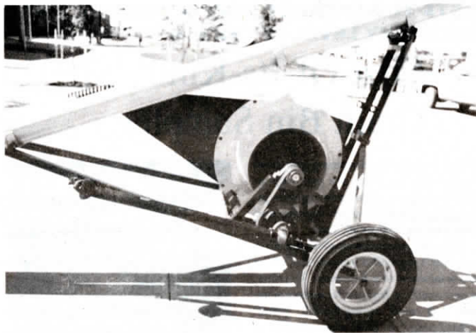
Blower delivers air, at rate of 1,460 cfm, down a 6-in. dia. tube to intake end of auger.
