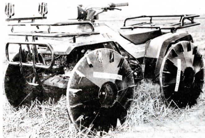
The 1-in. wide narrow steel wheels, which widen to about 6 in. at the hub, sink in only about 2 in. in mud.
