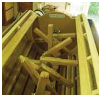
View shows beaters with loading section removed (left). Drum is covered with hardware cloth sized to allow peas through.
