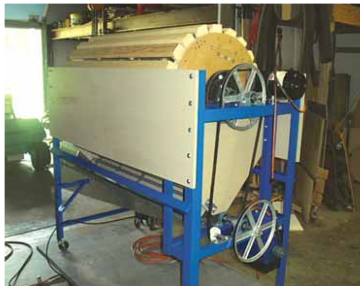
Ron Forster used wood and steel to build the beaters and drum on his pea sheller.
