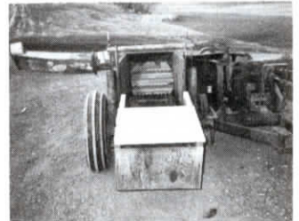
Leinbach built a wooden shelf over feed apron and turned blower pipe down to the side. He feeds papers by hand directly into chopper.
