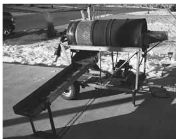
Larry Deglow came up with his own combination gold "trommel" and sluice box setup. It can go through 5 to 6 yards of dirt an hour.
