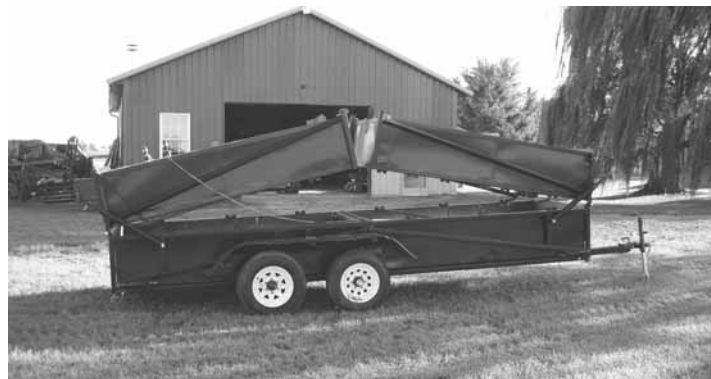
Trailer holds 2 stainless steel "pits", with wing pits hinged at either end that fold up for transport.
