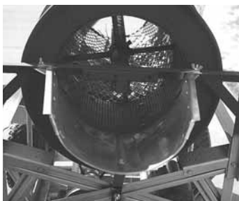
Outer drum consists of a 30-gal. barrel with a 13-in. wide, expanded metal screen positioned over the sluice.
