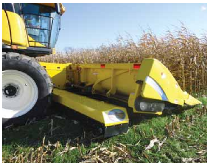
Cornrower uses rotating blades on each row to chop stover and send it to the center of combine, where it's deposited in a windrow machine.
