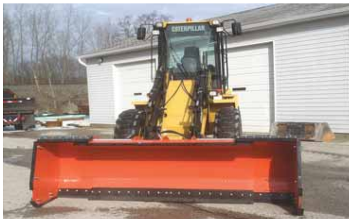
"Telescoping" loader bucket is equipped with two 2-ft. wide wings, each acted on by a hydraulic cylinder. Driver can move both wings in or out together, or separately.
