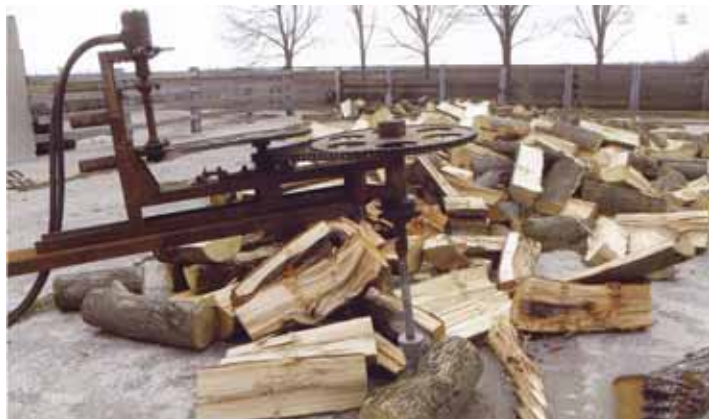
"It eliminates the need to do any lifting," says Garry Steeper, who built this 3-pt. mounted, hydraulic-operated screw-type log splitter using parts from an old barn gutter cleaner.
