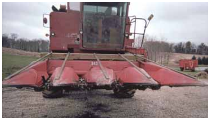
Miller bolted a treated wooden pole across top of header and then attached a series of 8 1/2-ft. long steel bars to pole. Opposite end of each bar is bolted onto snout.
