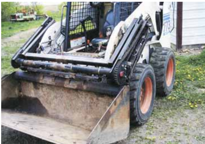
When it's not needed, grapple fork folds back out of the way against loader arms.
