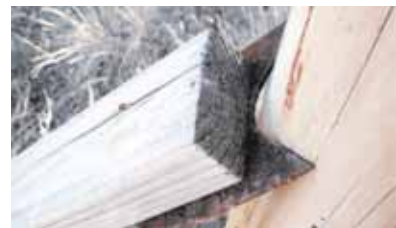
He pops the metal spades off old T-posts and then screws them to the ends of 2 by 4's.
