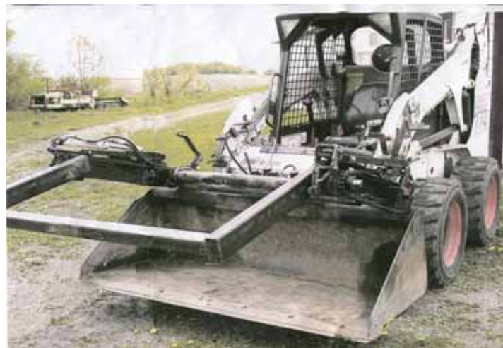
Grapple fork folds forward instantly when needed. Front bar can be fitted with teeth.
