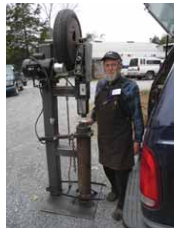
Unit is driven by a 1 hp, electric motor. Flat pulley mounted on motor rubs against tire to drive hammer downstroke.
