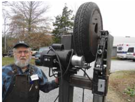
Tire Hammer is driven by an emergency spare tire mounted on a trailer axle and hub.
