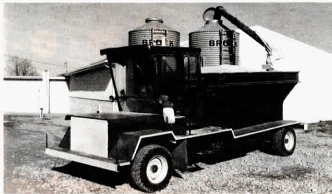
Cab on home-built feed truck, salvaged from an old Deere 55 combine, provides all-around visibility for lining up truck's auger with bins, feeders and bunks.
