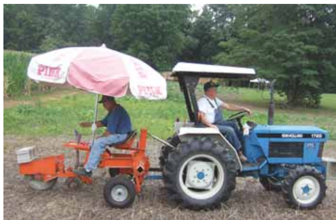
Terry Dunlap modified a single row Allis Chalmers no-till planter unit to make this one-row pumpkin planter, that he uses on his small pumpkin patch.
