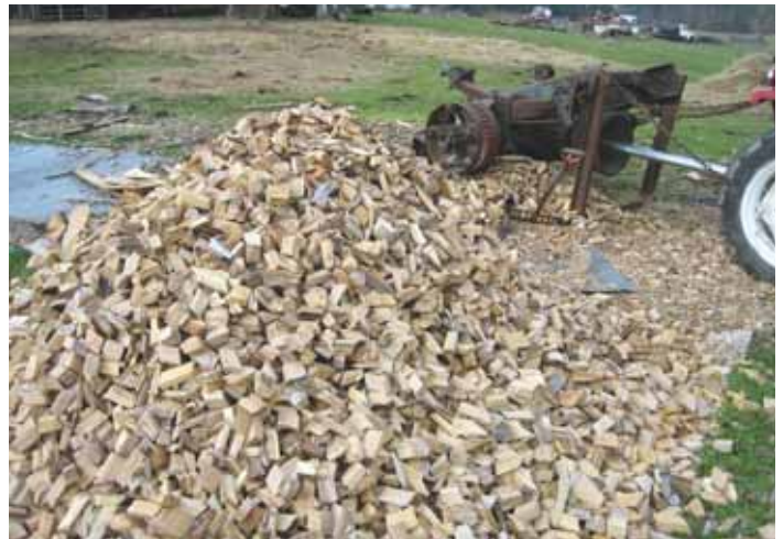
As chunks come off the machine, they’re scooped into piles for storage. Keith uses the little chunks of wood in his wood-powered trucks.
