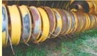
Baler pickup with bent, rusted steel bands.
