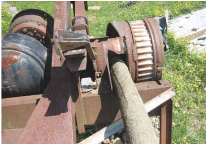
Wayne Keith designed this “chunker” that busts scrap wood into easy-to-handle pieces. Photo shows green wood being fed into chunker’s drum.
