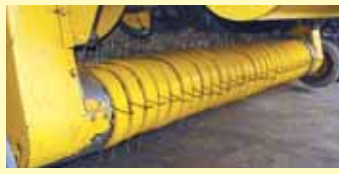
Pickup fitted with new Tobin poly bands.
