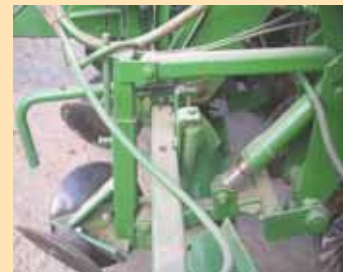
Hydraulics apply down pressure to crop rollers.
