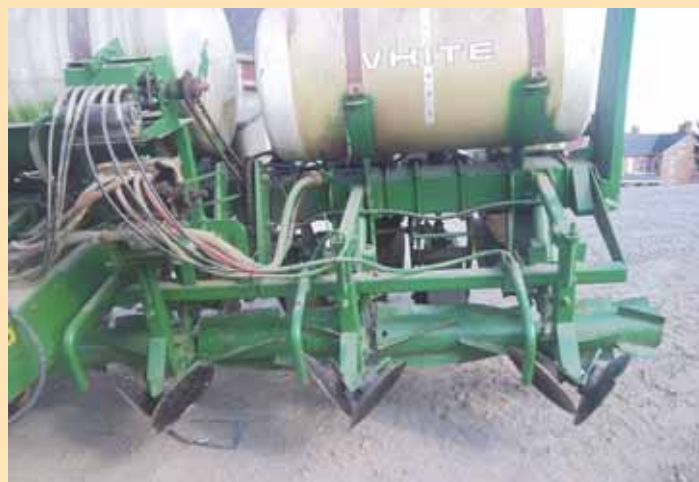
Charles Martin equipped his older Deere 7000 conservation planter, with a crop roller made from heavy steel pipe.
