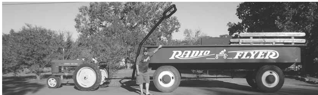
Texas-sized Radio Flyer wagon measures 7 ft. tall, 8 ft. wide and 20 ft. long and rides on the wheels off a semi truck. It was built on an old Deere running gear.
