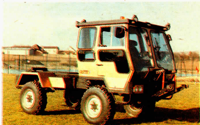
New Overtrack 100 features reversible operation, with both front and rear 3 pt. and pto.
