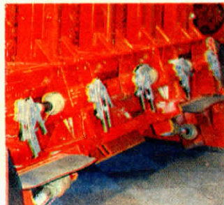
Flail-type stalk chopping knives on underside of a 6-row head for IH combines.
