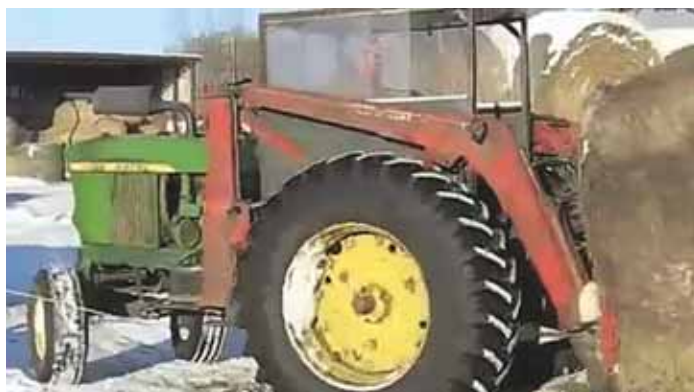
Ted Lacey flipped the differential, rear wheels, and operator station on his Deere 4020 tractor and mounted his Westendorf loader on back.
