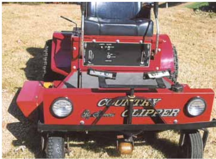
Gary Schultz added foot-operated steering controls to keep the front caster wheels from turning and drifting downhill on his zero turn riding mower.
