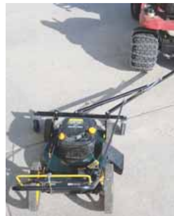
"Side kick" tow-behind mower attachment lets Tim Pickles pull a conventional push mower behind his riding mower.
