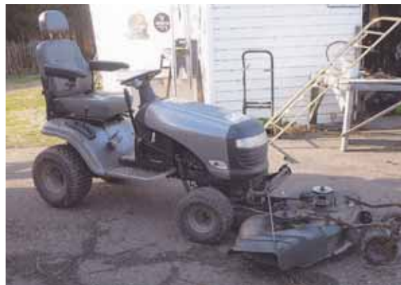
Front-mounted deck operates by pushing the up-and-down lever to engage the belt.
