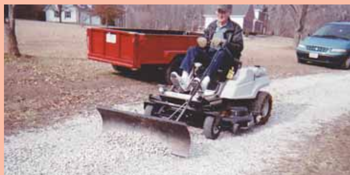
Vernon Foubert modified his new MTD Gold, 38-in. zero turn mower, adding a front-mount blade, a rear weight carrier, drive wheel chains, and foot pedals.
