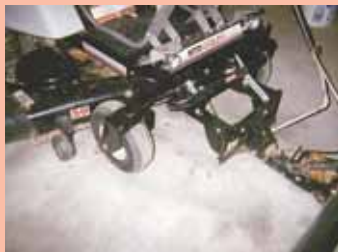
He added a bracket on mower's front frame to mount the blade.
