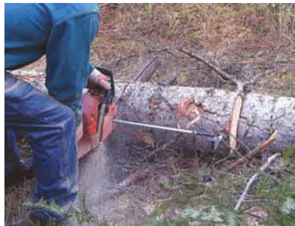
Telescoping guide rod attaches to chainsaw and is equipped with a battery-powered laser light. Operator lines up light with cut end of log and then starts sawing.
