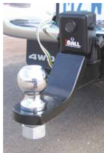
Battery-operated trailer hitch camera magnetically sticks to back of vehicle.
