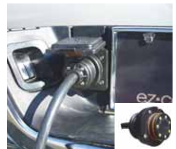
Magnetic trailer plug won't break if you forget to disconnect before driving away. Unit is waterproof and non-corrosive.
