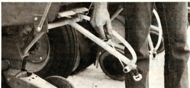
Bracket attaches to frame below planter boxes. Easily pivots for accurate placement.
