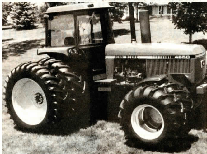
Add-on MFWD duals don't require alteration of frame.
