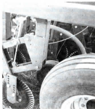
Each row unit consists of a fluted coulters and hoe opener followed by a press wheel.
