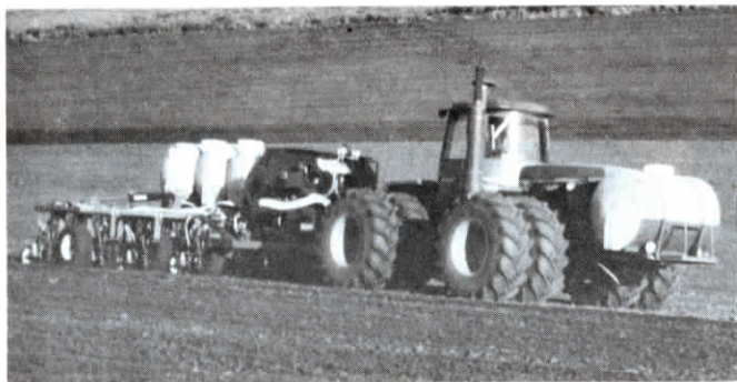
Drill supports two 500 gal. tanks and a 250 gal. tank. A 500 gal. tank also mounts on front of tractor.
