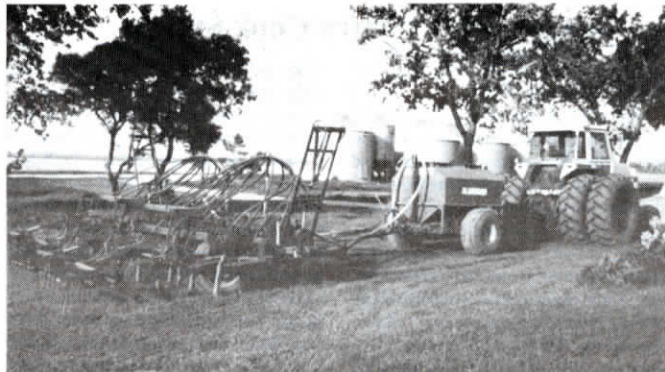
Bloomquist mounted two Morris drills together and pulls them behind a Blanchard air seeder, which carries 45 bu. of seed and 1,200 lbs. of fertilizer.
