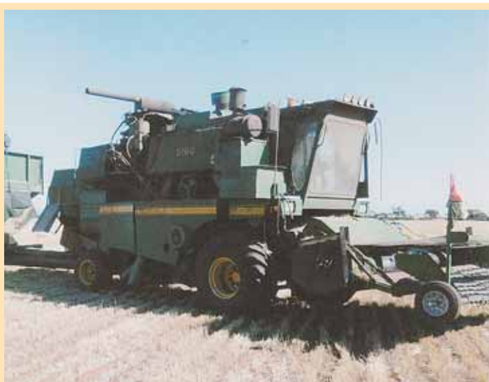
Malcolm Lucas of South Australia converted this German-built Fortschritt 5160 combine to electric power using off-the-shelf, 3-phase electric motors.
