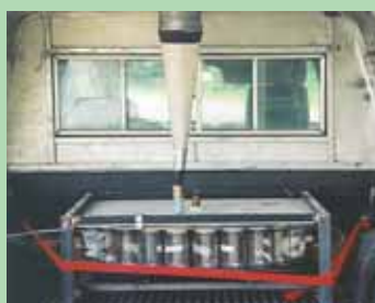
Captured insects drop through funnel into plastic bottles on carousel under pickup topper.
