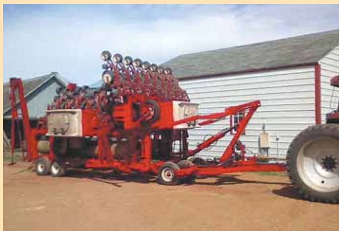
Folding the wings into transport position causes planter units to raise into a vertical position.
