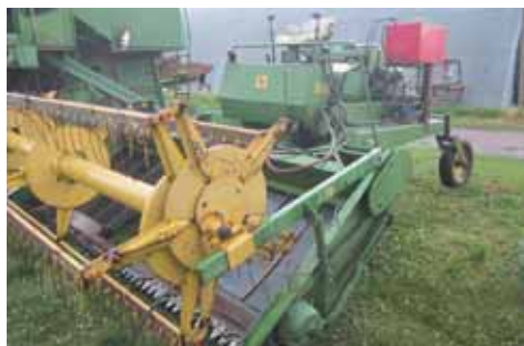
Add-on, self-contained hydraulic system controls the reel height and speed on this old Deere swather, which Bill Buman uses in his seed harvesting operation.
