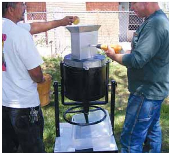
Gerald Simons redesigned his cider press and fruit cutter to bring the price down. Fruit cutter, mounted above press, can now be powered by electric drill.
