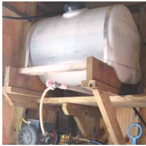
He mounted a 50-gal. soap tank above a pressurized water line, with soap solution gravity flowing to a soap injector.
