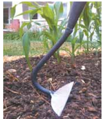
Hoe has an angled blade with a 7-in. wide edge that's beveled toward the user.
