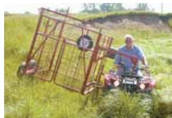
Calf Catcher attaches to front and rear of ATV and consists of a catch pen with spring-loaded gates. Operator opens the gates with a rope as he pulls up behind a calf.
