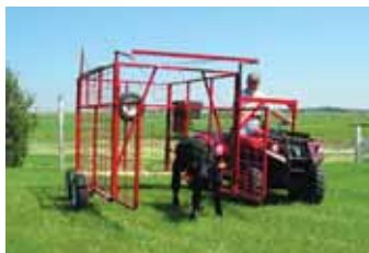
Calf Catcher attaches to front and rear of ATV and consists of a catch pen with spring-loaded gates. Operator opens the gates with a rope as he pulls up behind a calf.
