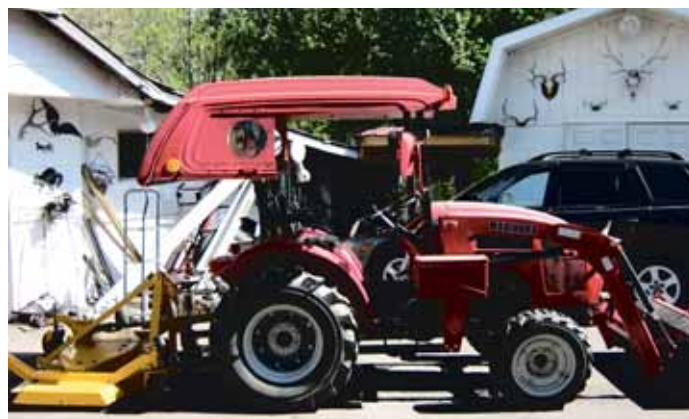
James Bohn used the fiberglass topper off an old Chevy S-10 pickup to make this canopy for his Mahindra 25 hp loader tractor.
