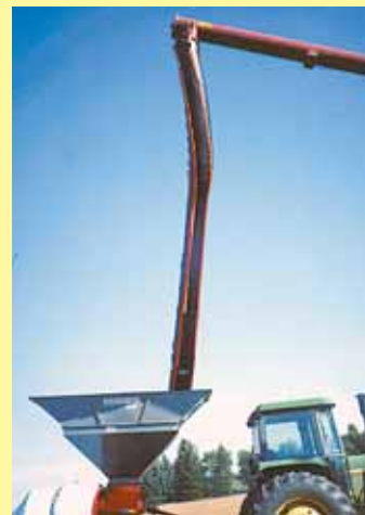
The 30-ft. flexible spout extension makes it easier to fill grain bagger with an auger and semi truck, instead of having to use a smaller grain cart or tandem axle truck.
