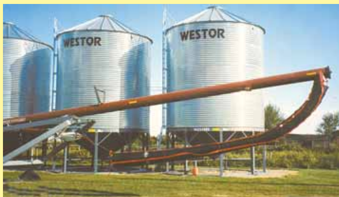
The 30-ft. flexible spout extension makes it easier to fill grain bagger with an auger and semi truck, instead of having to use a smaller grain cart or tandem axle truck.
