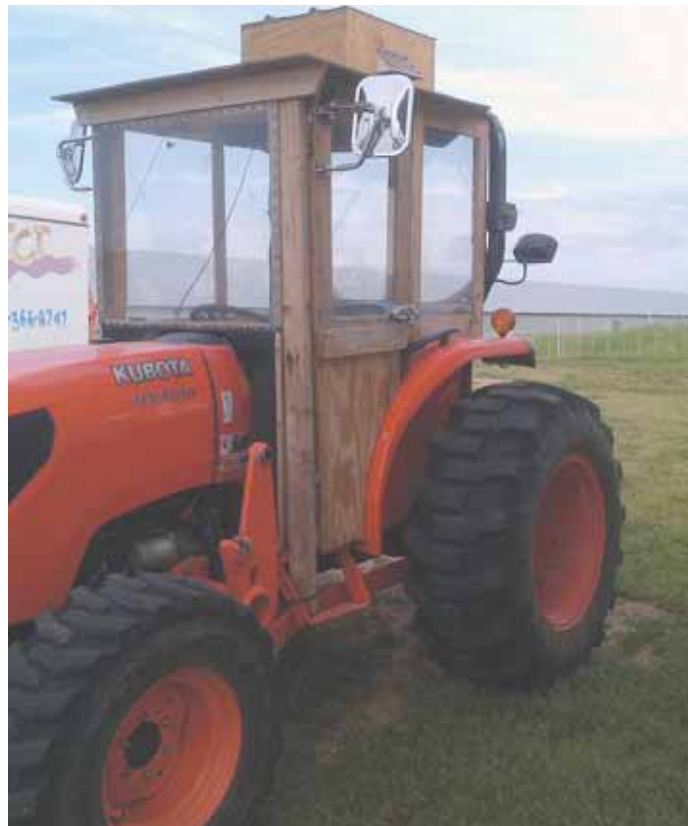
John Headings used 1/4-in. plywood to make this cab for his Kubota 51 hp 4-WD tractor. Blower fan on top of cab helps him stay cool during summer.
