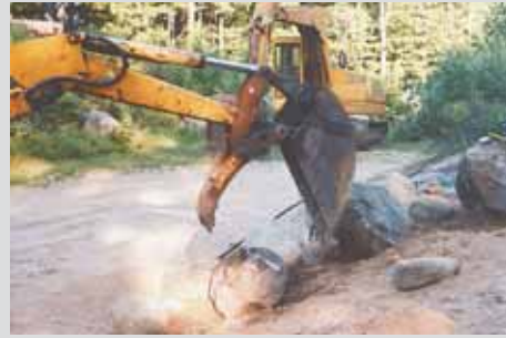
Hoe Clamp moves as bucket moves. Lund says it’s easier to use than a “hydraulic thumb”.
