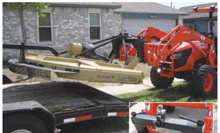
Steven Rios converted a Cat. I, 3-pt. quick hitch into this skid steer-style attachment. "It lets me hook up an implement and load it without having to get off the tractor," he says.
