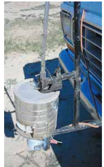
Jeff Hoard made a broadcast spinner/seeder from a large coffee can and other scrap materials and then strapped it on front of his pickup.
