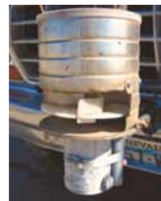
Plastic propeller mounts at bottom of coffee can and is powered by a 12-volt fan motor mounted below.
