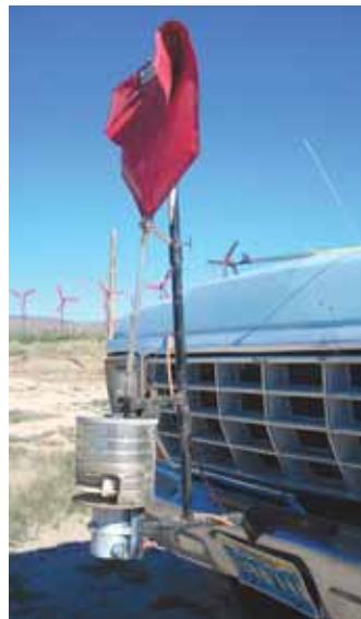
Jeff Hoard made a broadcast spinner/seeder from a large coffee can and other scrap materials and then strapped it on front of his pickup.
