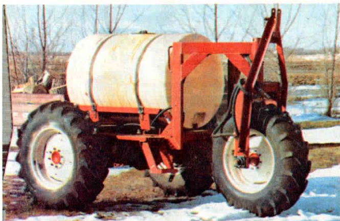
Andrew Schuelke's 3-wheel caddy carries a 500 gal. tank and a roller pump.
