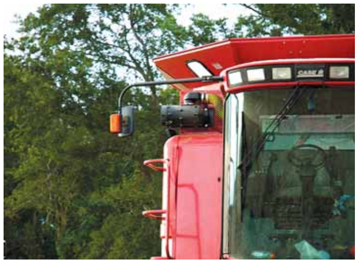
Sy-Klone’s high-tech filtering system provides ultra-clean air to machinery operators, in part by pressurizing the cab.
