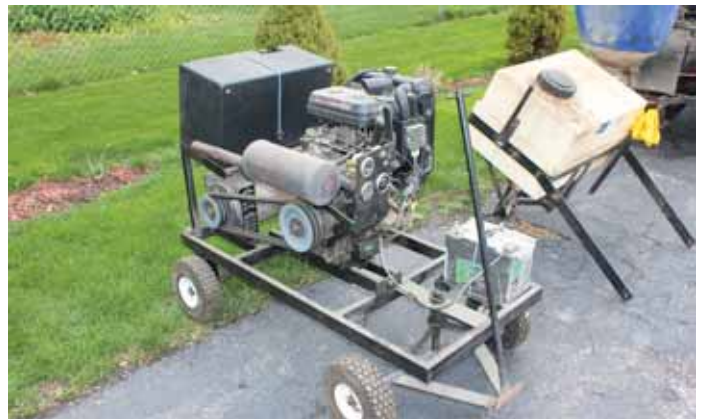
Frank Orr built this low-cost portable generator using the 22 hp engine off a riding mower. Twin belt pulleys on both engine and alternator provide increased rpm’s.
