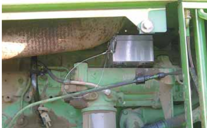
Sheldon Sivak’s manifold-mounted lunch box produces a warm meal even when the weather is cold. Magnets on bottom of box hold it tightly against any hot metal surface.
