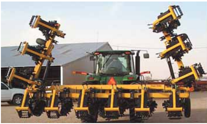
Chopper Stalker uses razor-sharp blades and rolling disks to cut and size corn stalks. It's designed to be used at a field speed of 8 to 10 mph.
