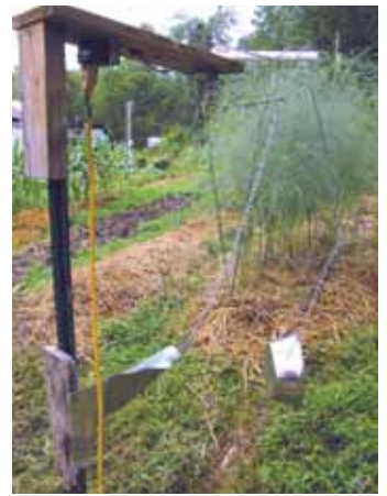
Rotating drive arm causes golf ball to strike a sheet of tin and make a vibrating sound. Then ball swings into a stainless steel pan, creating a metallic ringing sound.
