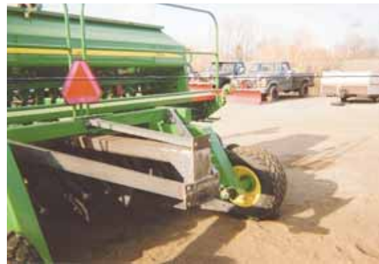
Anyone wanting to roll fields behind their drill can get help from Adelmeyer Welding, which fabricates heavy duty hitches to match drill frames.
