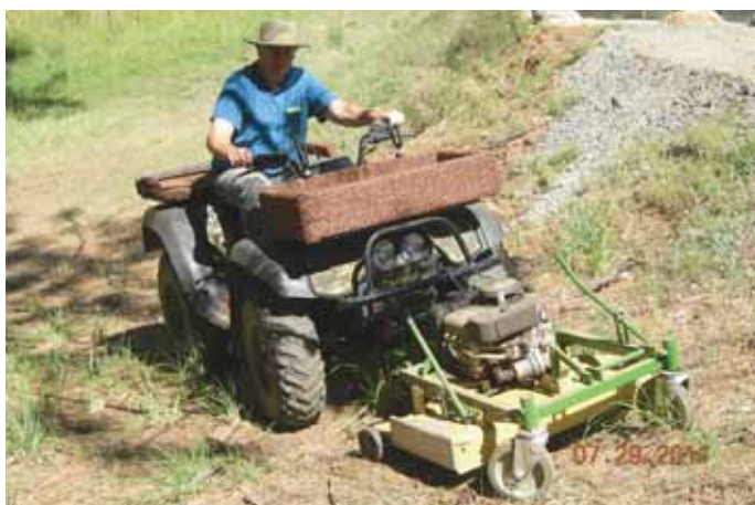
Gale Wells mounted a 36-in. deck off a Deere riding mower on front of his Suzuki 4-WD ATV, adding an 8 hp Briggs & Stratton engine to power it.
