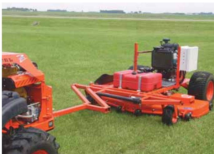
Variable-width, offset mower is designed to be pulled by a riding mower, 4-wheeler or utility tractor. All operations are remote-controlled from the vehicle pulling it.
