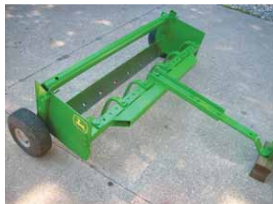
Steve Nichols' homemade box scraper, complete with scarifier shanks, is designed to be pulled behind a garden tractor.
