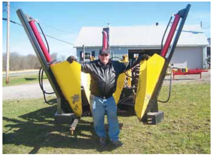
David Sager built his own tree spade, mounting it on his loader's quick-tach hitch.
