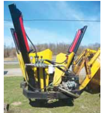
A 6 hp motor and hydraulic pump is used to drive each of the spade's 3 cylinders separately.
