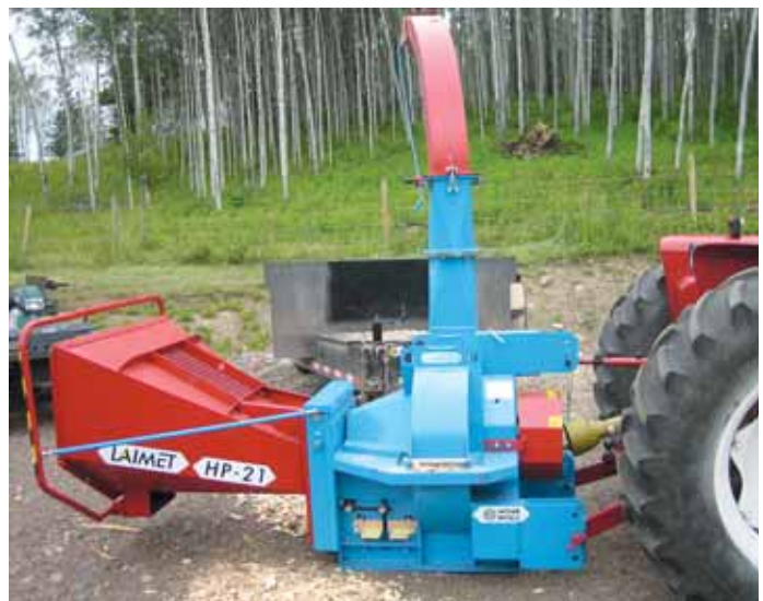
Pto-powered wood chipper from Finland lets customers select from 8 different screw blades and 5 different chip sizes, between 1/2 in. and 4 in. in length.
