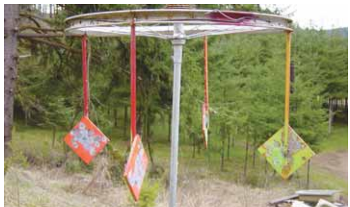
"Revolving" rifle target spins on the hub of an ordinary bicycle wheel, propelled by the force of the bullets hitting the diamond-shaped metal targets.
