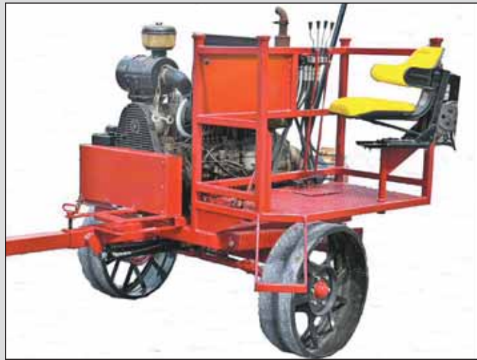
Horse-drawn power unit can be used for cutting, raking and baling hay, as well as chopping silage, and many other farm jobs that require tractor-like power.
