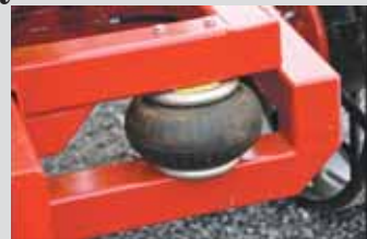
Unit is fitted with air bag shock absorbers and dual hydraulic outlets powered by a gas or diesel engine.
